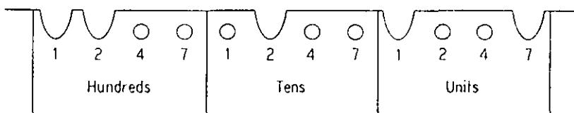
To select the card with number 328 from the stack, one or more needles could be used. If two needles are used, they would be placed in the '1' and '7' units holes and the cards which fall would be re-sorted by inserting one needle in the '2' tens hole; finally, by placing needles in the '1' and '2' hundreds holes of the fallen cards, only cards with the number 328 will drop out.
